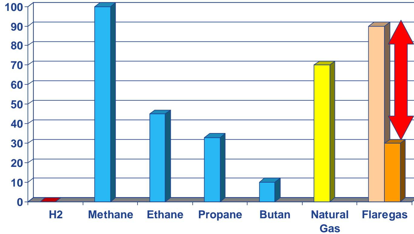
**Methane Number is the main limiting factor for the achievable output of Flare gas Applications**
