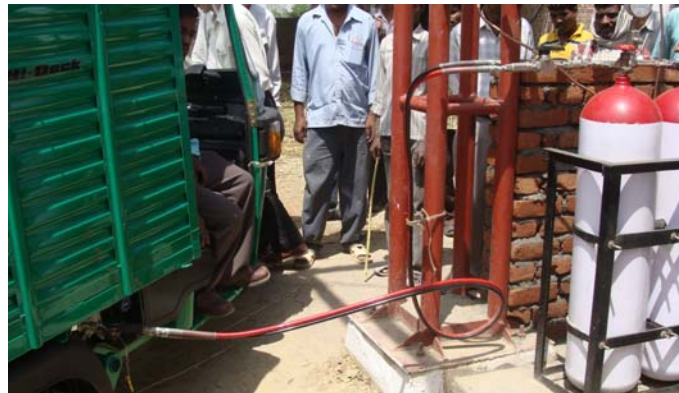
Enriched Bio-Gas cylinders dispensing gas in Vehicle
