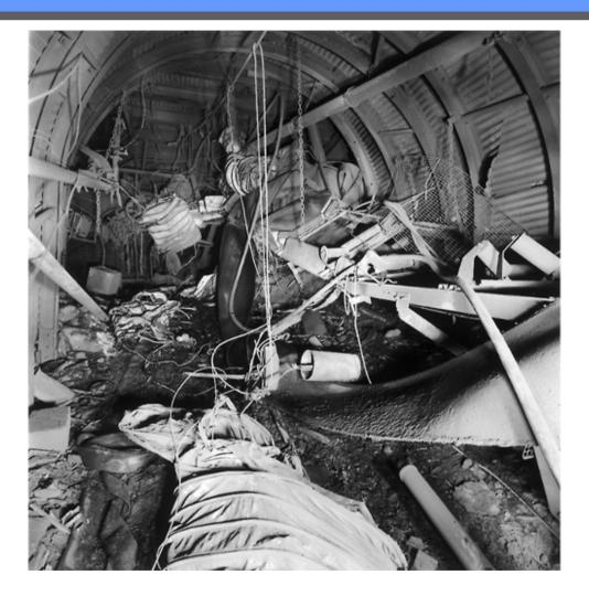
CMM ignited when drawn over live switchgear - Killing 10
