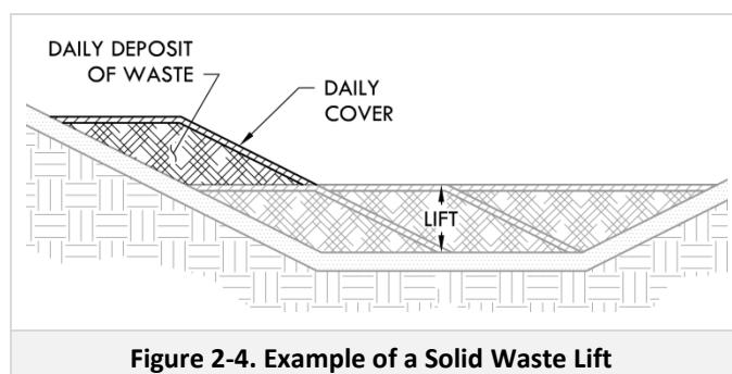
Figure 2-4. Example of a Solid Waste Lift
