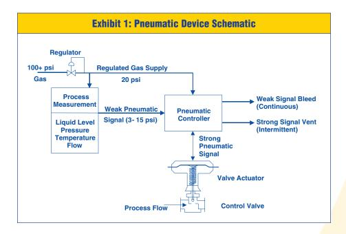
In general, controllers of similar design usually have similar steady-state bleed rates regardless of brand name. Pneumatic devices come in three basic designs:
