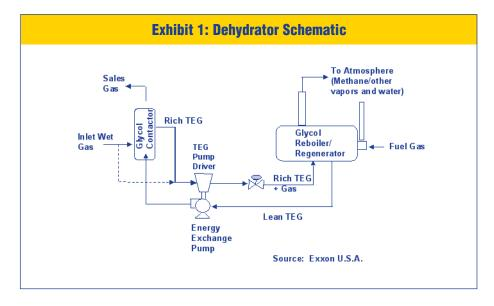
pumps increase emissions from dehydrator systems by passing the pneumatic driver gas entrained with rich TEG to the reboiler. A basic overview of the pump's operation is described below:
