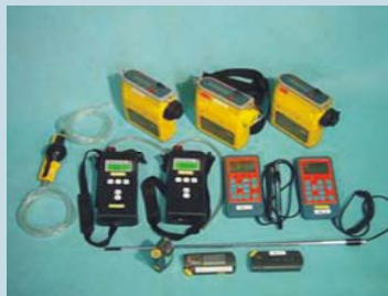
Leakage detectors, methane concentration meters
