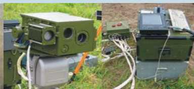
Board passive distant gas meter for methane concentration "Tomsk-1"
