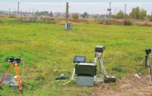
Distant measuring system of methane concentration
