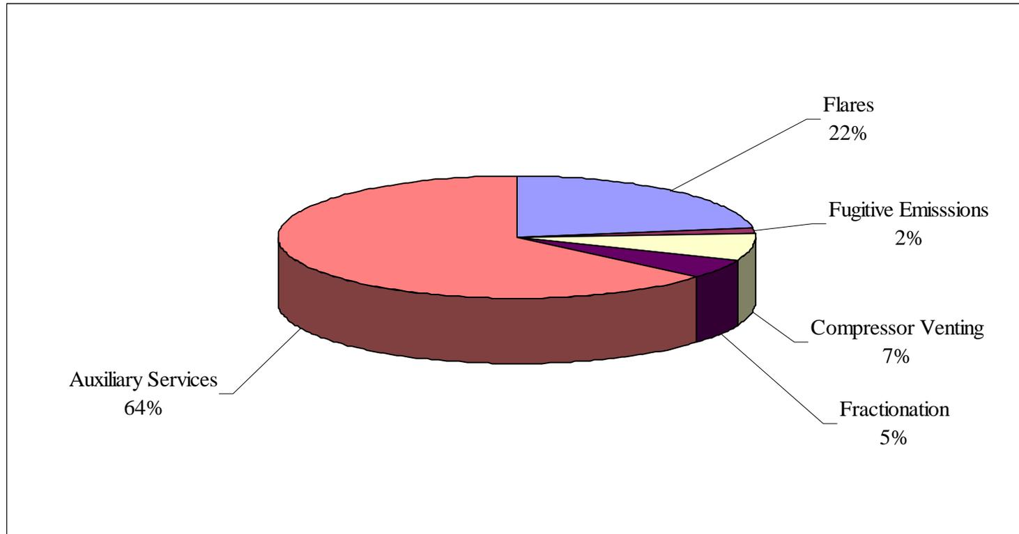
*These values are based on gas volumes vented, fugitive emissions in equipment and components, and inefficiency in combustion equipment measured during the field work.*
