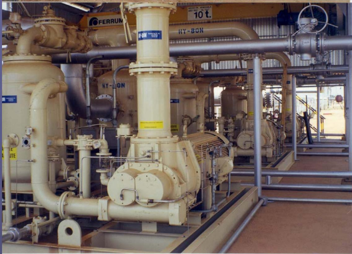
*At this location, three of our compressor packages were set in tandem to move 15 MMSCFD of 2500-2600 BTU tank vapors.*
