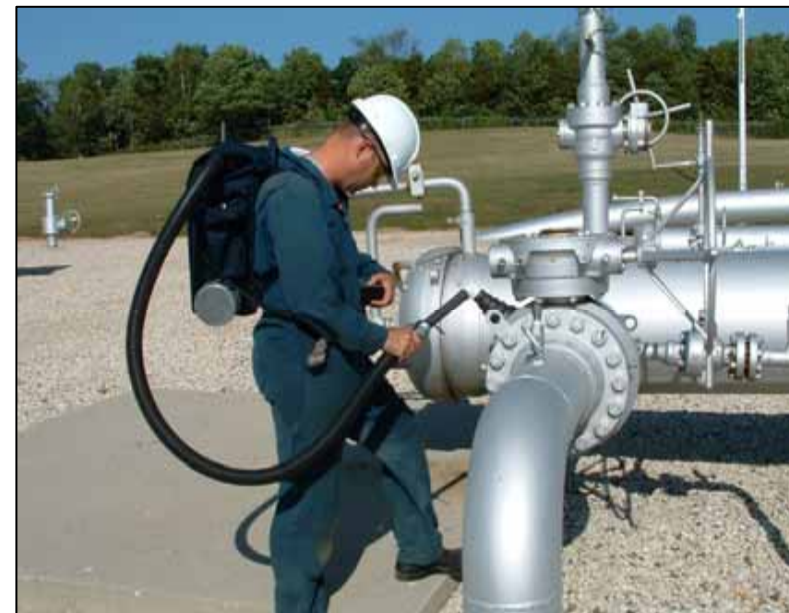
Leak Measurement Using High Volume Sampler 用大容积取样器测量泄漏
