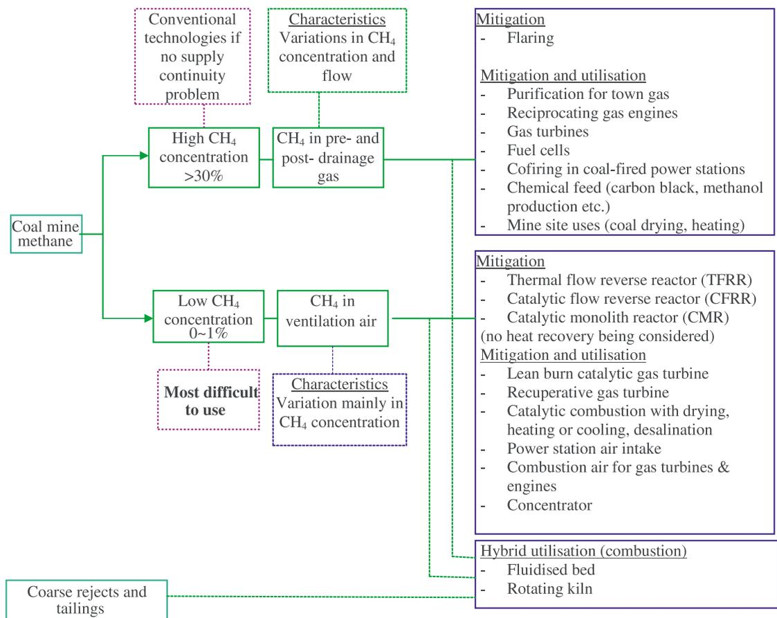
Fig. 1. Illustration of classifying mine methane mitigation and utilisation technologies.
