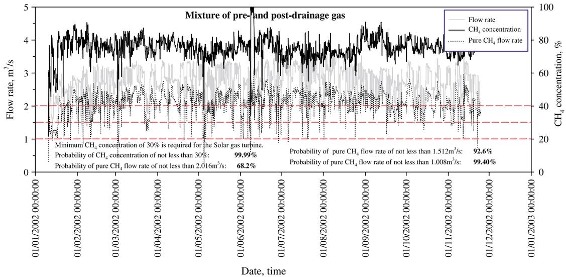
Fig. 12. Potential of the conventional gas turbine power generation plant at the QLD mine.
