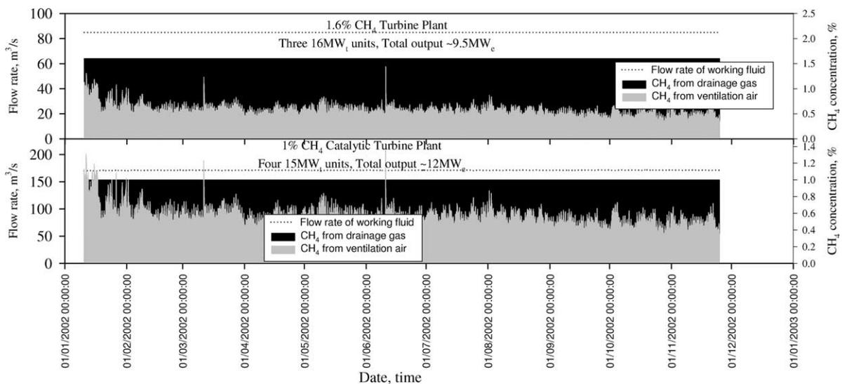
Fig. 18. Operating states of the 1 and 1.6% methane turbine plants at the QLD mine.
