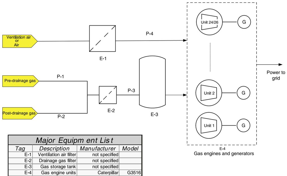
Fig. 8. Diagram of internal combustion gas engine power generation system at the QLD mine.
