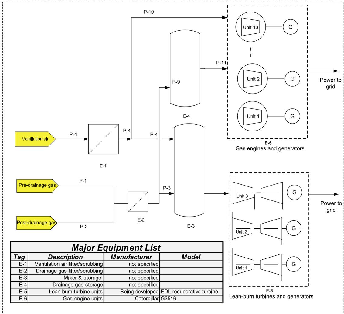
Fig. 23. Diagram of the combined 1.6% methane turbine and gas engine power generation system at the QLD mine.
