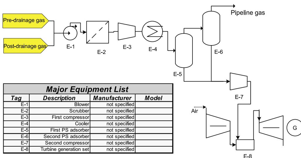
Fig. 7. Diagram of a typical process for pressure swing adsorption purification of gas.
