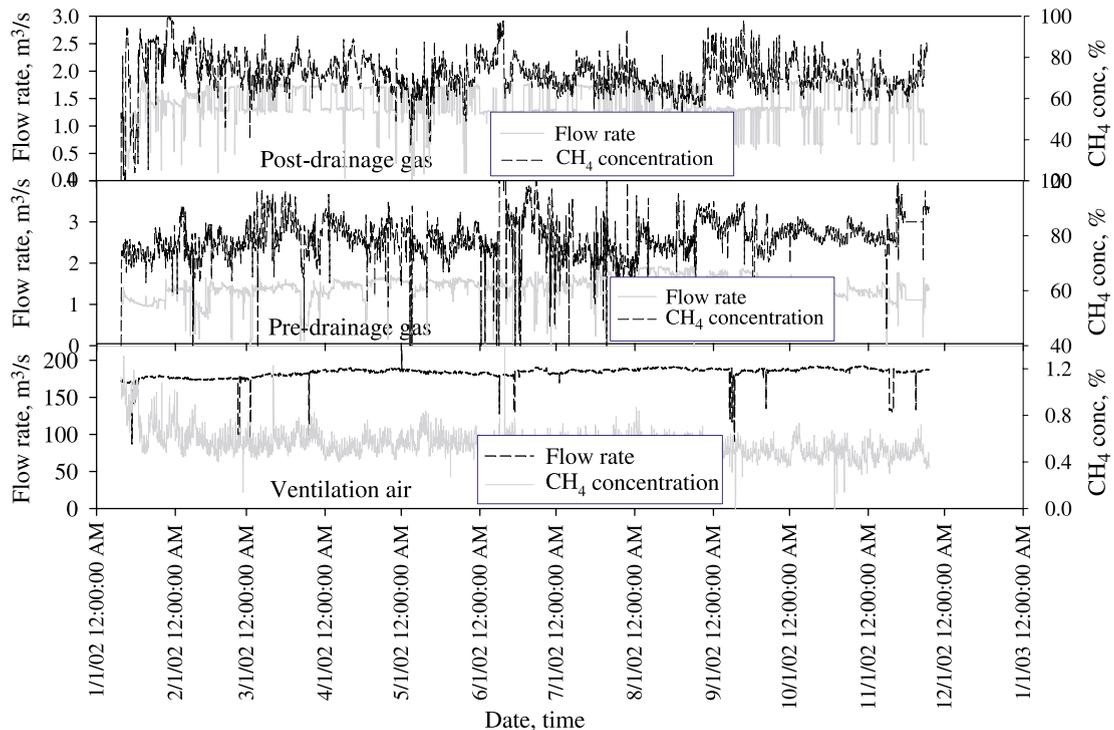
Fig. 6. Characteristics of methane emissions from a Queensland mine.
