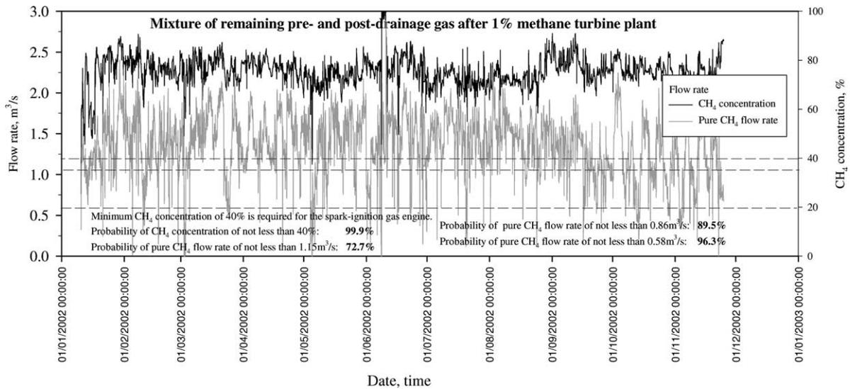
Fig. 19. Potential of the gas engine power generation plant after the 1% methane turbine plant at the QLD mine.
