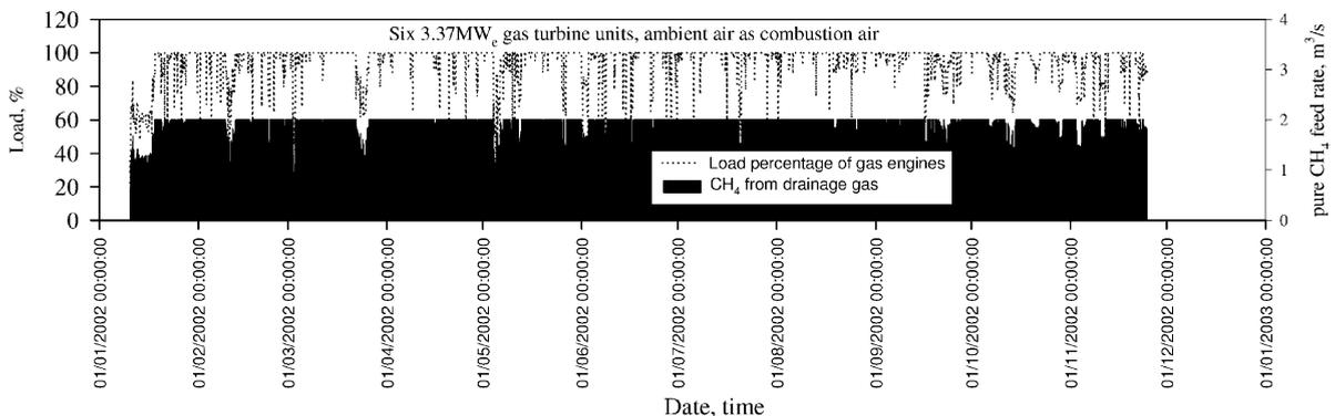
Fig. 13. Operating state of the conventional gas turbine power plant at the QLD mine.
