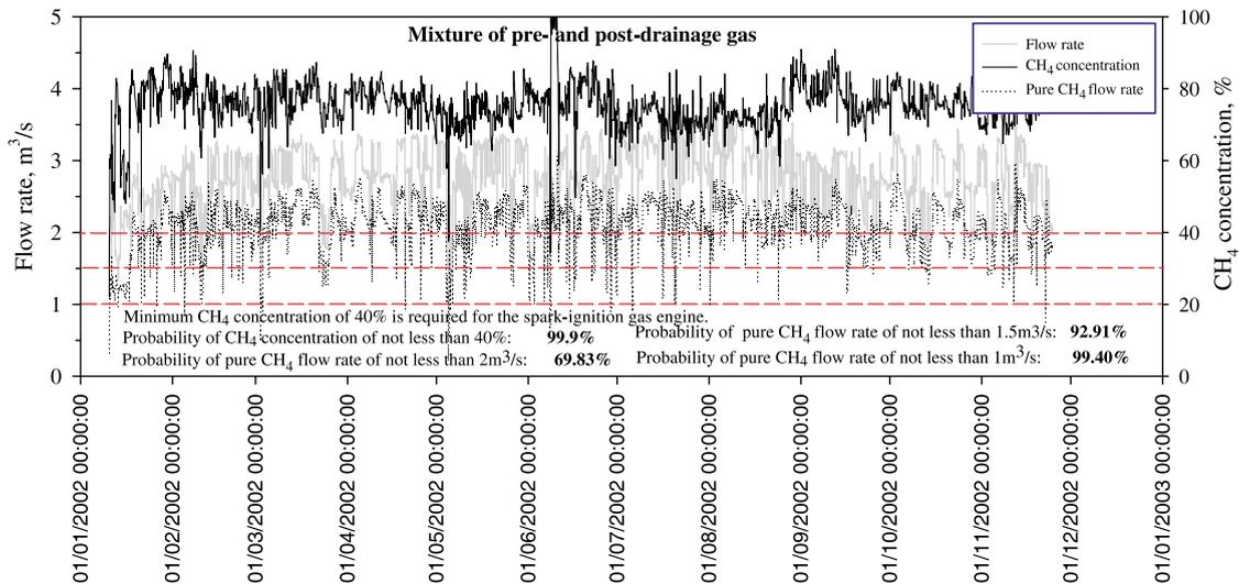
Fig. 9. Potential of the gas engine power generation plant at the QLD mine.
