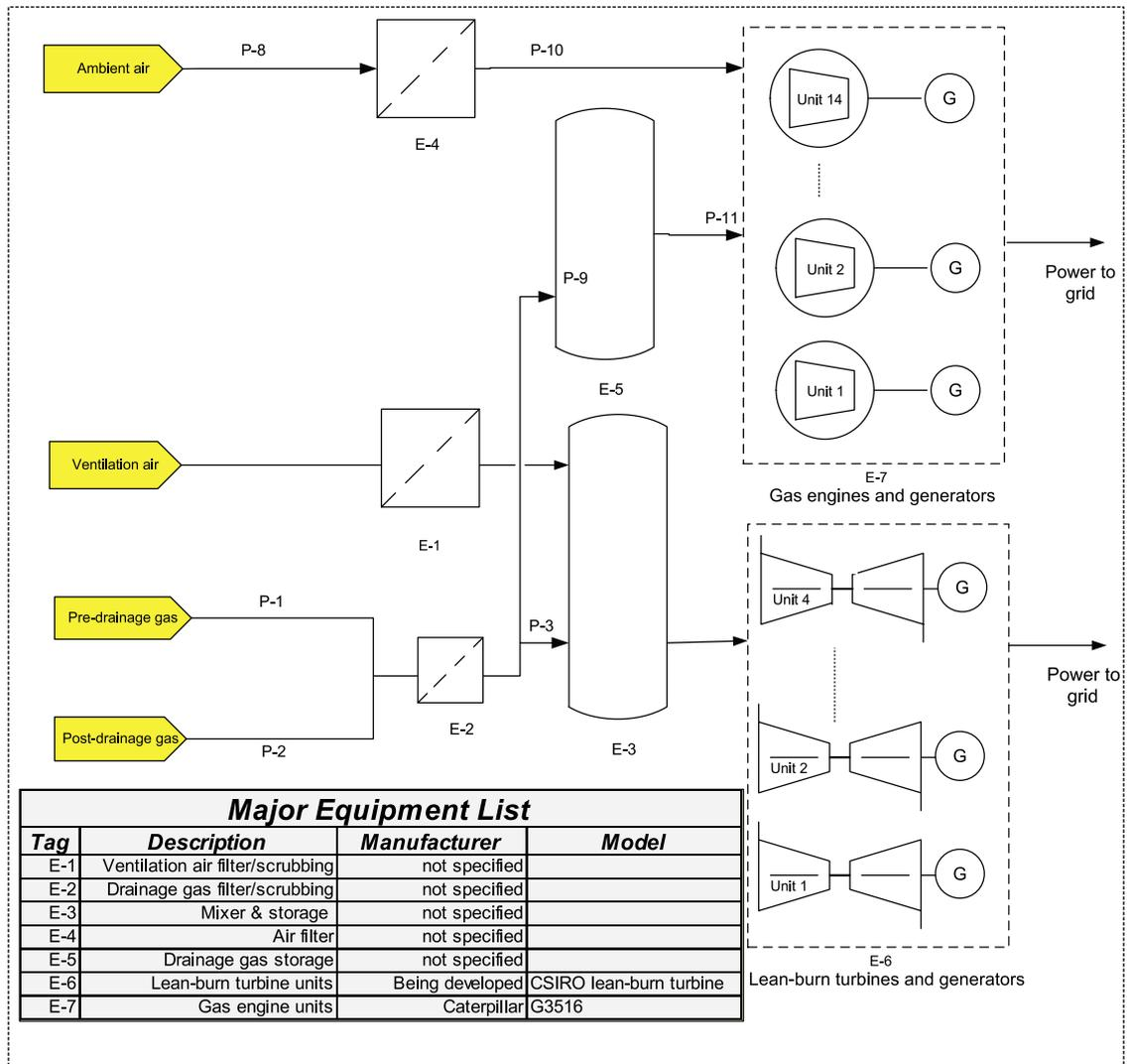
Fig. 20. Diagram of the combined 1% methane turbine and gas engine power generation system at the QLD mine.
