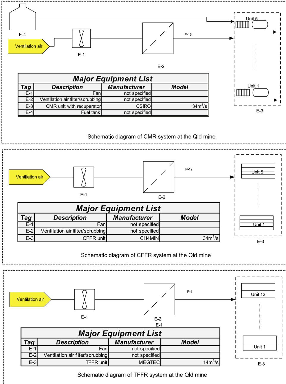
Fig. 15. Diagram of TFFR, CFFR or CMR methane mitigation plant system at the QLD mine.
