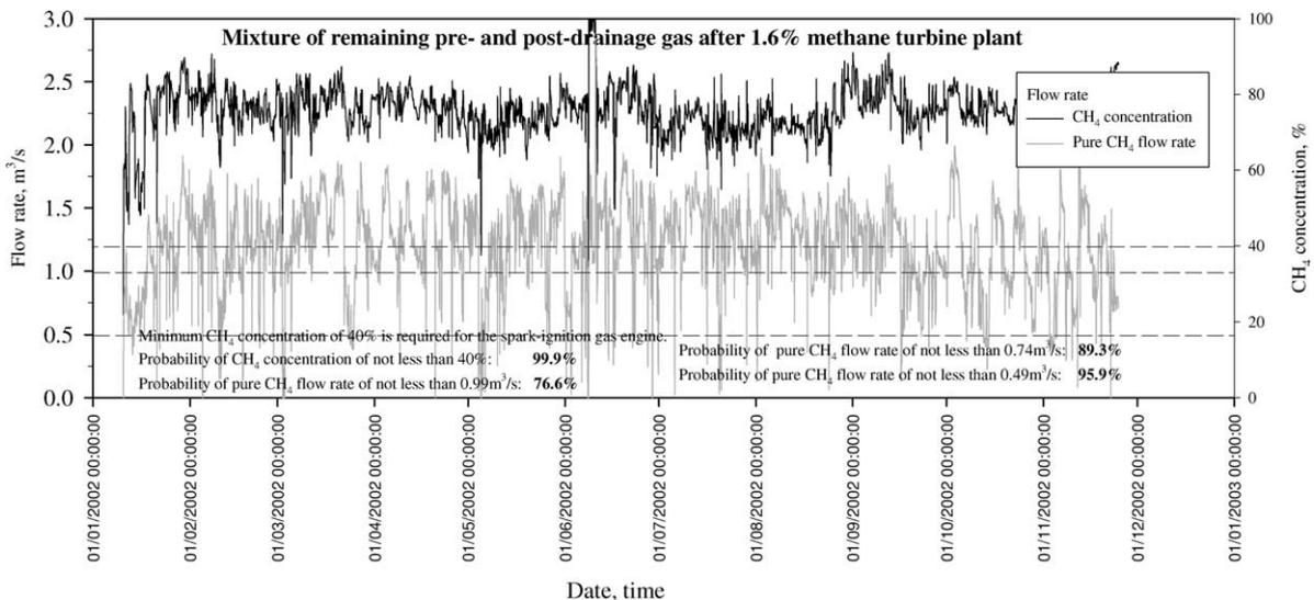
Fig. 22. Potential of the gas engine power generation plant after the 1.6% methane turbine plant at the QLD mine.
