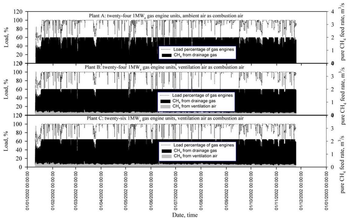
Fig. 10. Operating state of the gas engine power plant at the QLD mine.
