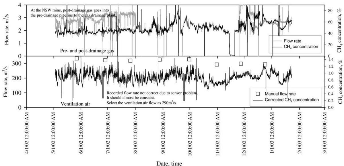
Fig. A1. Characteristics of methane emissions from the NSW coal mine.
