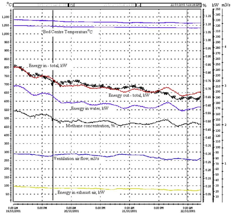
Fig. 5. TFRR test unit operating chart (extracted from [38]).
