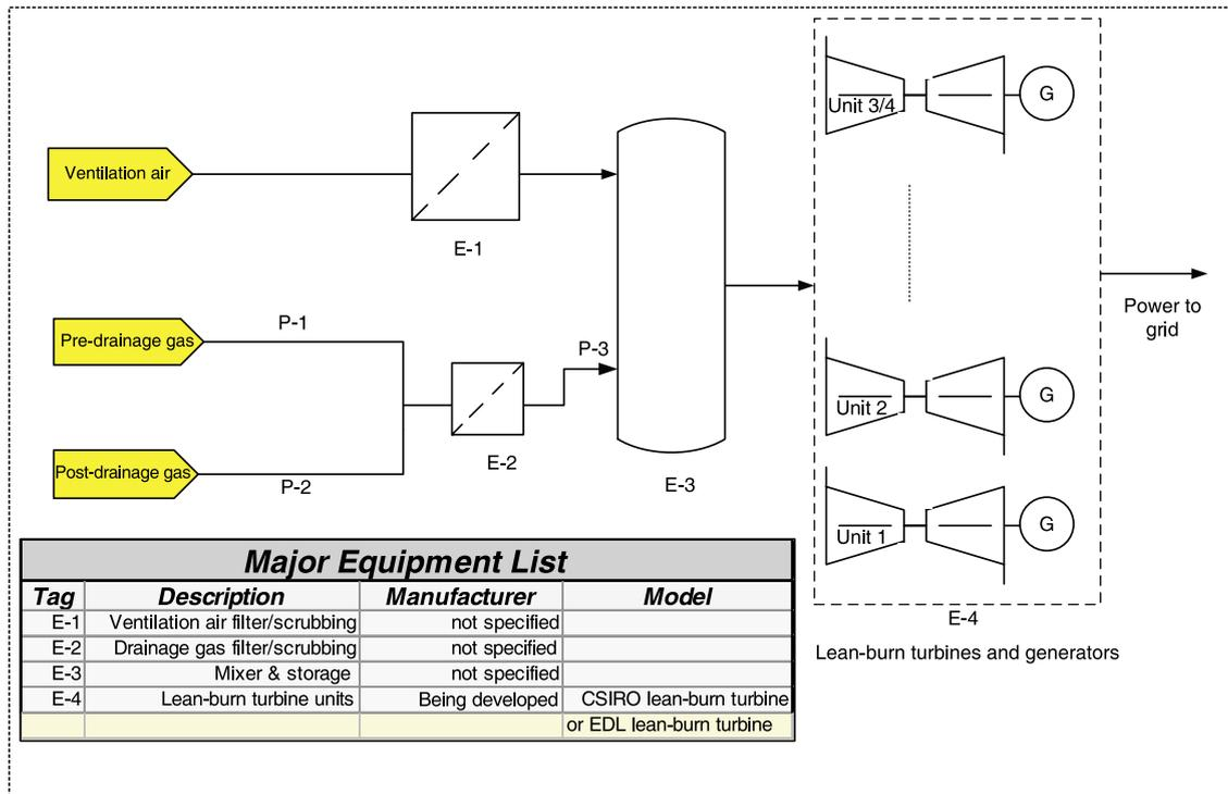
Fig. 17. Diagram of CSIRO or EDL lean-burn gas turbine plant at the QLD mine.
