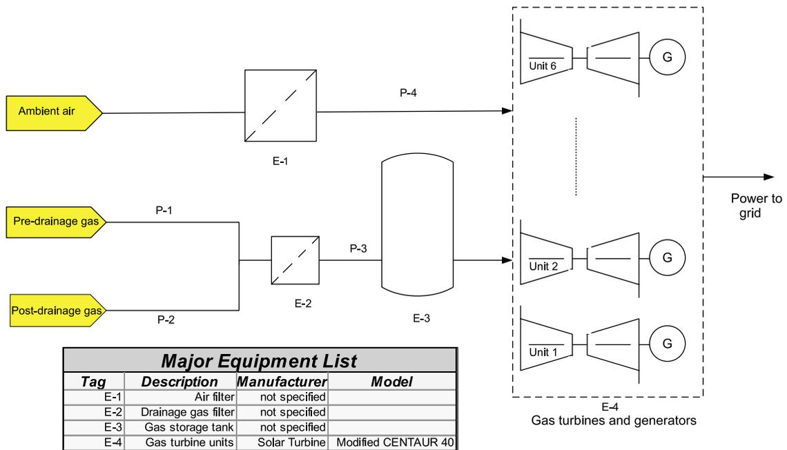
Fig. 11. Diagram of CENTAUR 40 gas turbine power generation system at the QLD mine.
