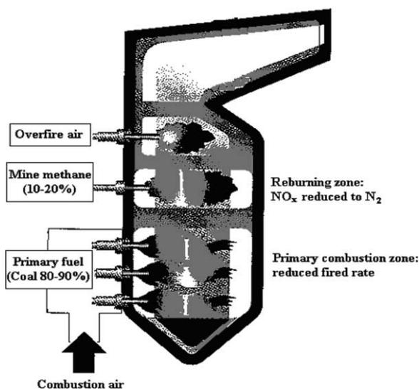
Fig. 2. Principle of reburning technology (modified from [24]).
