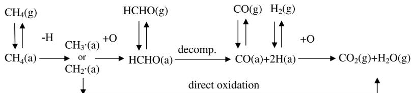
Fig. 4. A possible mechanism for methane catalytic oxidation [31]: (a) adsorbed, (g) gas phase.
