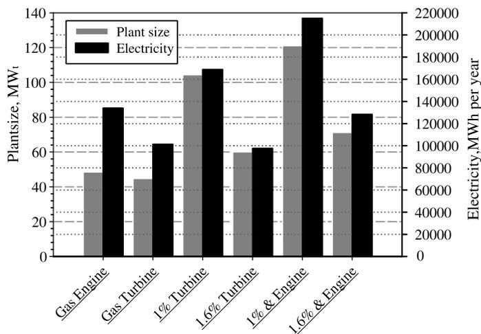
Fig. A2. A comparison of plant sizes and electricity production at the NSW mine.
