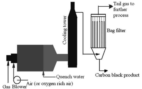
Fig. 3. A simplified diagram of the semi-reinforcement gas furnace carbon black production technology [28].
