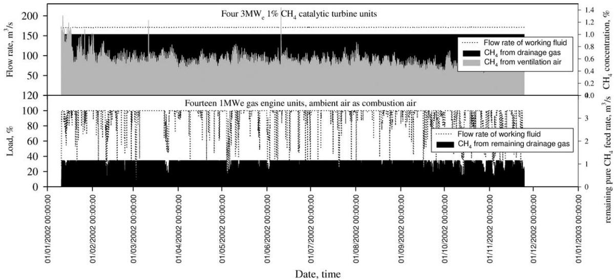
Fig. 21. Operating state of the combined 1% methane turbine and gas engine power plant at the QLD mine.
