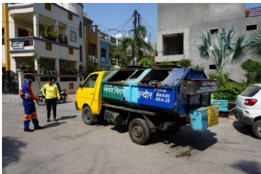
Figure 4: A collection vehicle with separate chambers for dry, wet, and hazardous waste.
