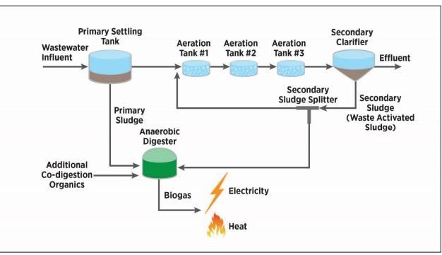
Typical Conventional Activated Sludge Plant with Anaerobic Digestion
