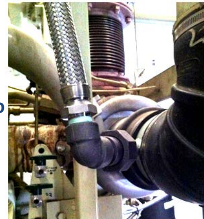
SlipStream® gas injection point to engine
