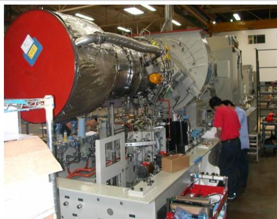
**Figure 4-7: Dual Gas Wide Wobbe Fuel Assembly and Fuel Injectors on a Solar LFG Turbine<sup>13</sup>**
