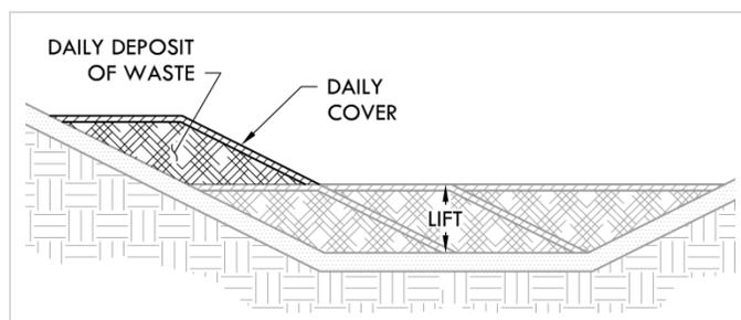
Figure 2-4. Example of a Solid Waste Lift
