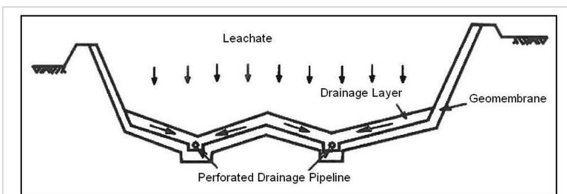
Figure 2-2. Side View of Leachate Drainage Slopes
