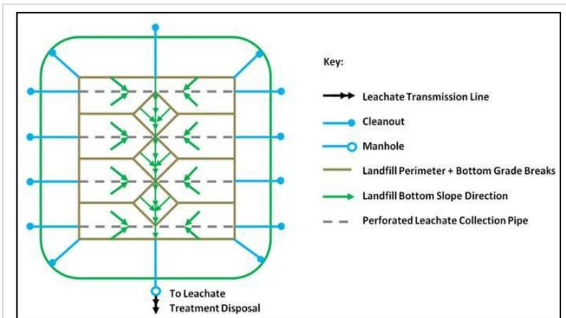
Figure 2-1. Typical Layout of Leachate Collection System (top view)
