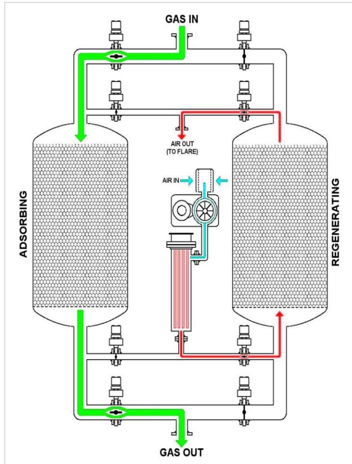
Figure 4-10. Diagram of the a siloxane removal system
