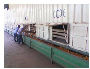
Inclined Bed Corn-on-cob Dryers
