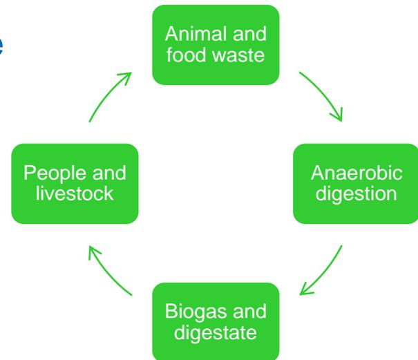
**Biogas** is a mixture of methane, carbon dioxide and water and can be used to produce electricity and heat or used as a natural gas substitute.
