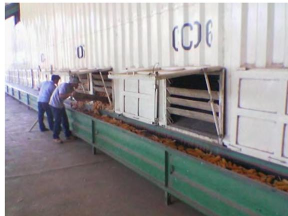
Inclined Bed Corn-on-cob Dryers
