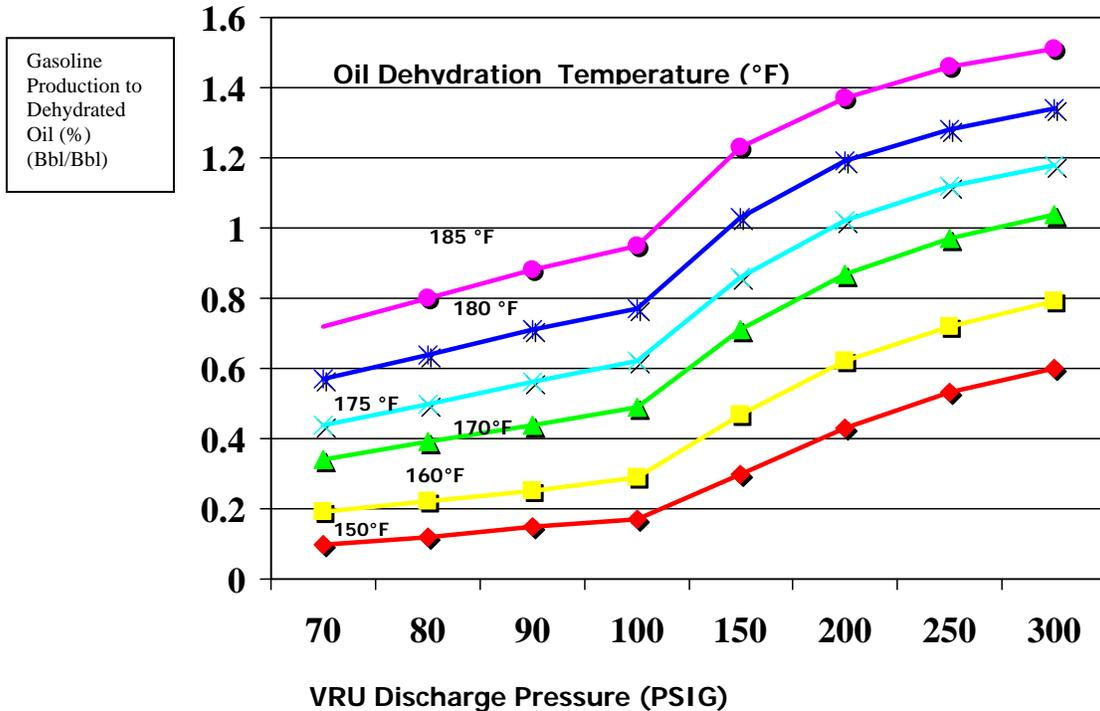
The Vapor Recovery Units allow optimizing the relationship between crude oil variables like chemical injection and Dehydration Temperature. Without the VRU, all light fractions evaporated in tanks are directed to the vent, resulting in economical losses.
