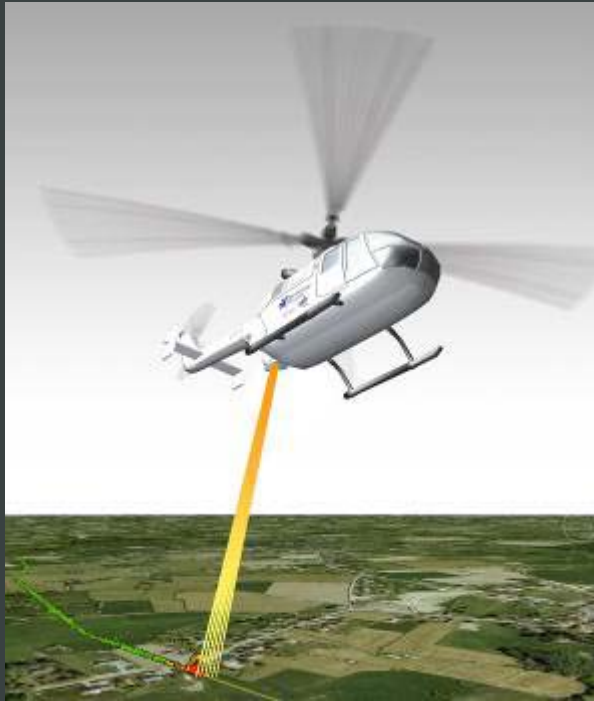
CHARM® for buried pipelines (active principle)
