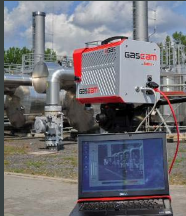
GasCam® for above ground installations (passive method)
