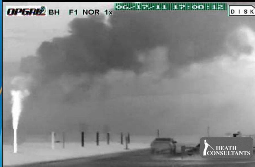
Compressor Station Blow Down Normal Mode
